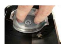
Remove the clear plastic cap from the top of the fill can. Press the metal reservoir cup on top of the can with the smallest opening resting on the top of the fill can. Slide the cap into the metal reservoir cup, so that it mates with the bottom of the cup. Using your index finger, press the bottom of the plastic cap into the bottom of the reservoir cup to ensure a snug fit.
