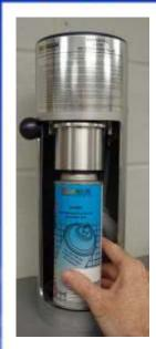
Gently place the reservoir and can into the filling machine, keeping them connected at all times. Slide the brim of the reservoir cup into the reservoir slot. Rotate the black base counterclockwise to snug the connection between the can and cup. Close door.
